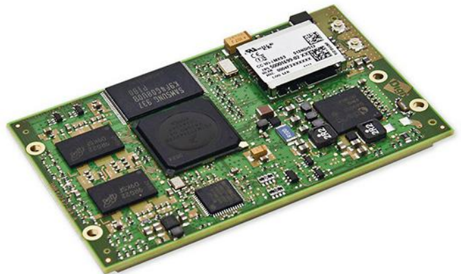
1. Digi International's ConnectCore i.MX53/Wi-i.MX53 runs NXP's i.MX8, which is able to handle machine-learning chores.
