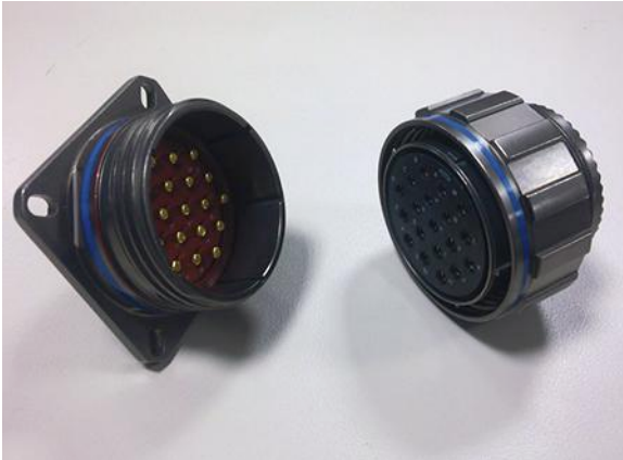
The MIL-DTL-38999 nickel plated polymer connector is designed for use in rugged environments. (Source: Abailleul via Wikipedia)
