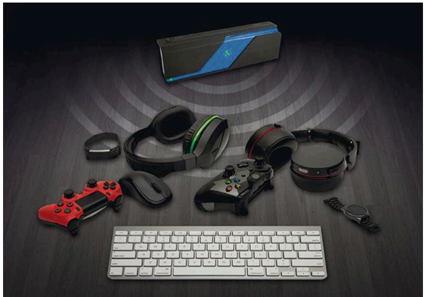
3. The PowerSpot long-range charger by Powercast creates a charging zone up to 80 feet away, accommodating the charging of multiple devices.
